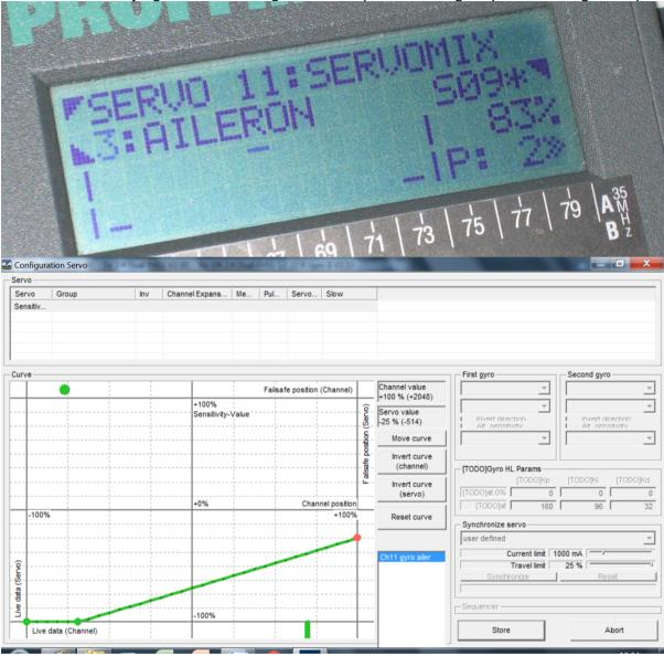
Now if you watch GigaControl while switching the retracts up and down with the aileron stick at centre you will see that the horizontal control marker jumps left and right, thus altering the gain for the different flight conditions.
