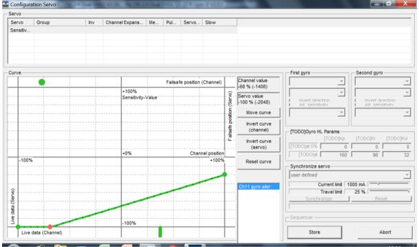
That establishes the value for normal flight and for the purpose of this illustration we will assume that the landing gain is some arbitrary higher value. This time we do not need to bother too much about the gain value on the vertical axis, because we need to program the Tx aileron stick to replicate the position of the green control bar on the horizontal axis. Make a careful note of its position as that is what we need to replicate a little later.
